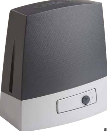
**BKX** is the most advanced and powerful sliding motor, with brushless 24 V DC motor and native encoder, ideal for residential and industrial gate applications up to 1200 kg.
